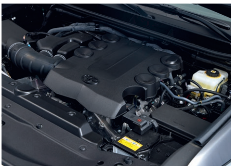
4.0L 1GR-FE GAS ENGINE WITH 275 PS AND 381 NM TORQUE
